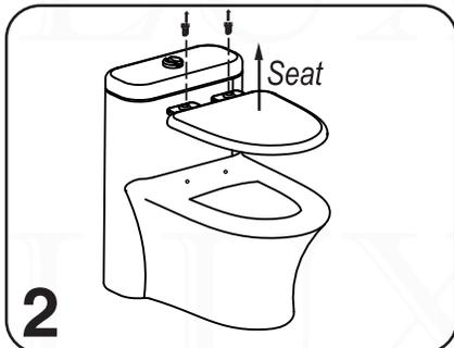
**2** Remove the seat by unscrewing the seat.
