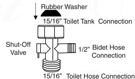
This metal t-adaptor has a shut-off valve to limit or cut off cold water to the bidet. It can be used instead of the plastic t-adaptor for the cold water connection.
