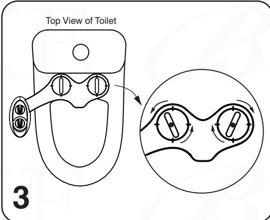
**3** Place the bidet on the toilet. Plates may be adjusted depending on where the two holes in the back of the toilet are.
