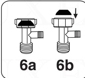
**6a:** Make sure that there is a black rubber washer inserted at the top of the t-adapter.
